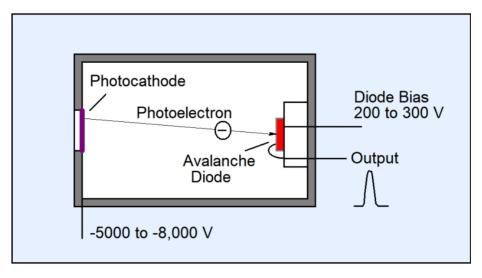
When an electron hits the avalanche diode it generates a large number of electron-hole pairs in the silicon. These carriers are further amplified by the linear gain of the avalanche diode. The total gain is on the order of  $10^6$ , i.e. sufficient to generate a detectable current pulse at the output of the avalanche diode.
