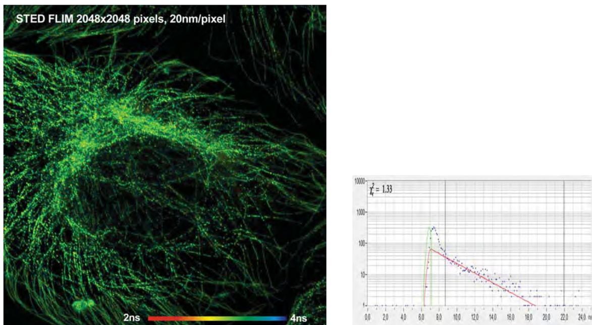
Fig. 32: STED FLIM with Abberior Instruments STED microscope. 2048 x 2048 pixels. Single cell, stained with tubulin-binding dye, recorded at a resolution of 20 nm per pixel. Decay curve in selected pixel shown on the right. The initial peak is undepleted fluorescence. It is gated off in the intensity data of image shown on the left.
