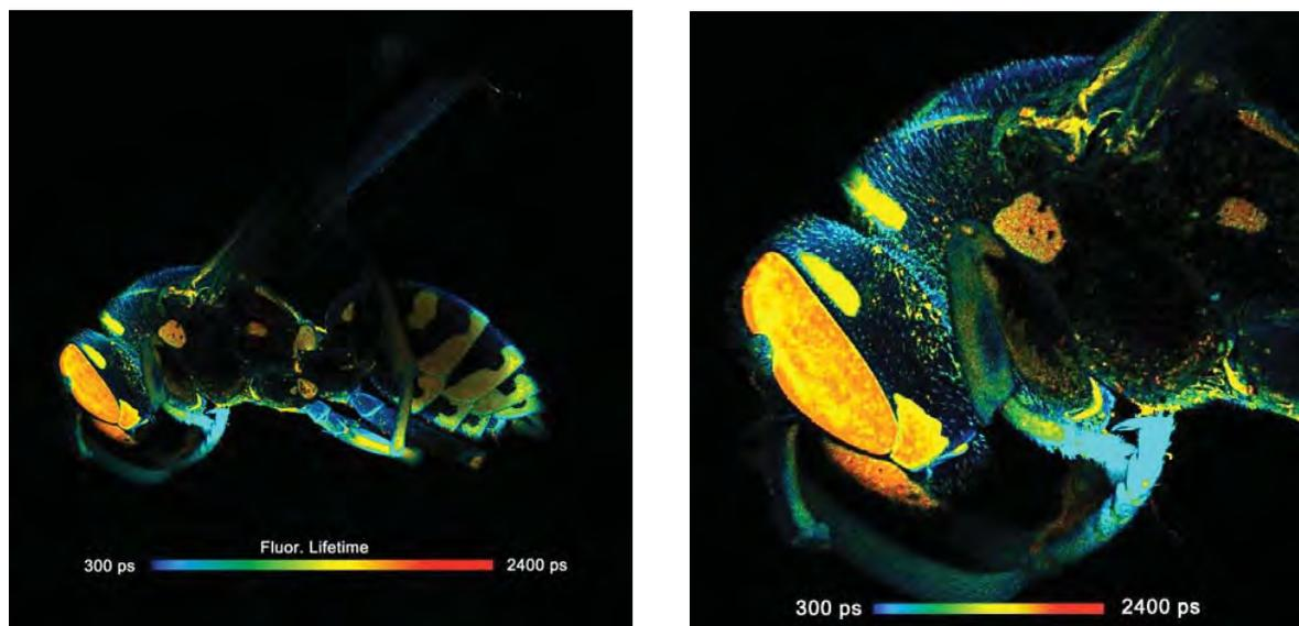
Fig. 30: FLIM of a macroscopic object. Resolution 2048 x2048 pixels, 256 time channels. Left: Original image. Right: digital zoom into recorded FLIM image, showing the excellent resolution of the data.
