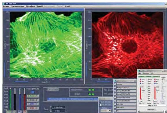
Fig. 9: SPCM software in fast preview mode. 1 image per second, two parallel FLIM channels recording in separate wavelength intervals.
