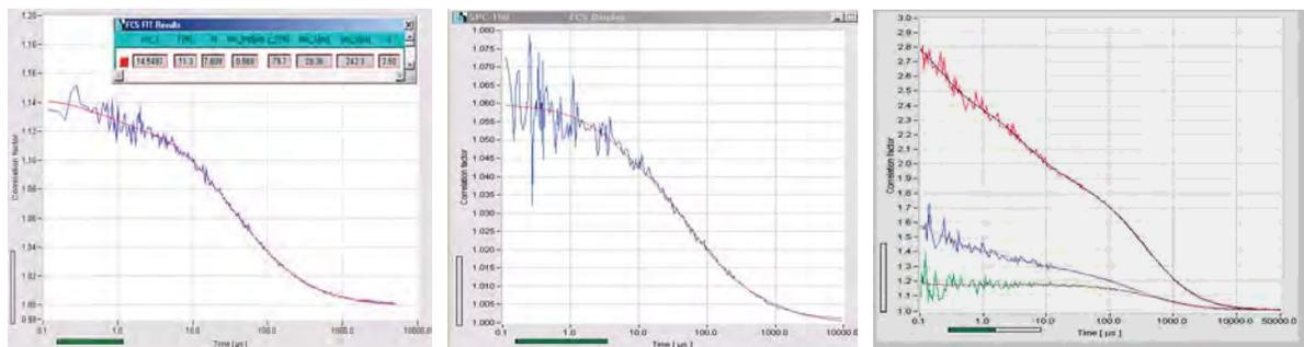
Fig. 33: FCS with bh TCSPC FLIM systems, GaAsP hybrid detectors. Left to right: Confocal FCS with ps diode laser, two-photon NDD FCS, cross correlation of photons recorded in different detection channels.
