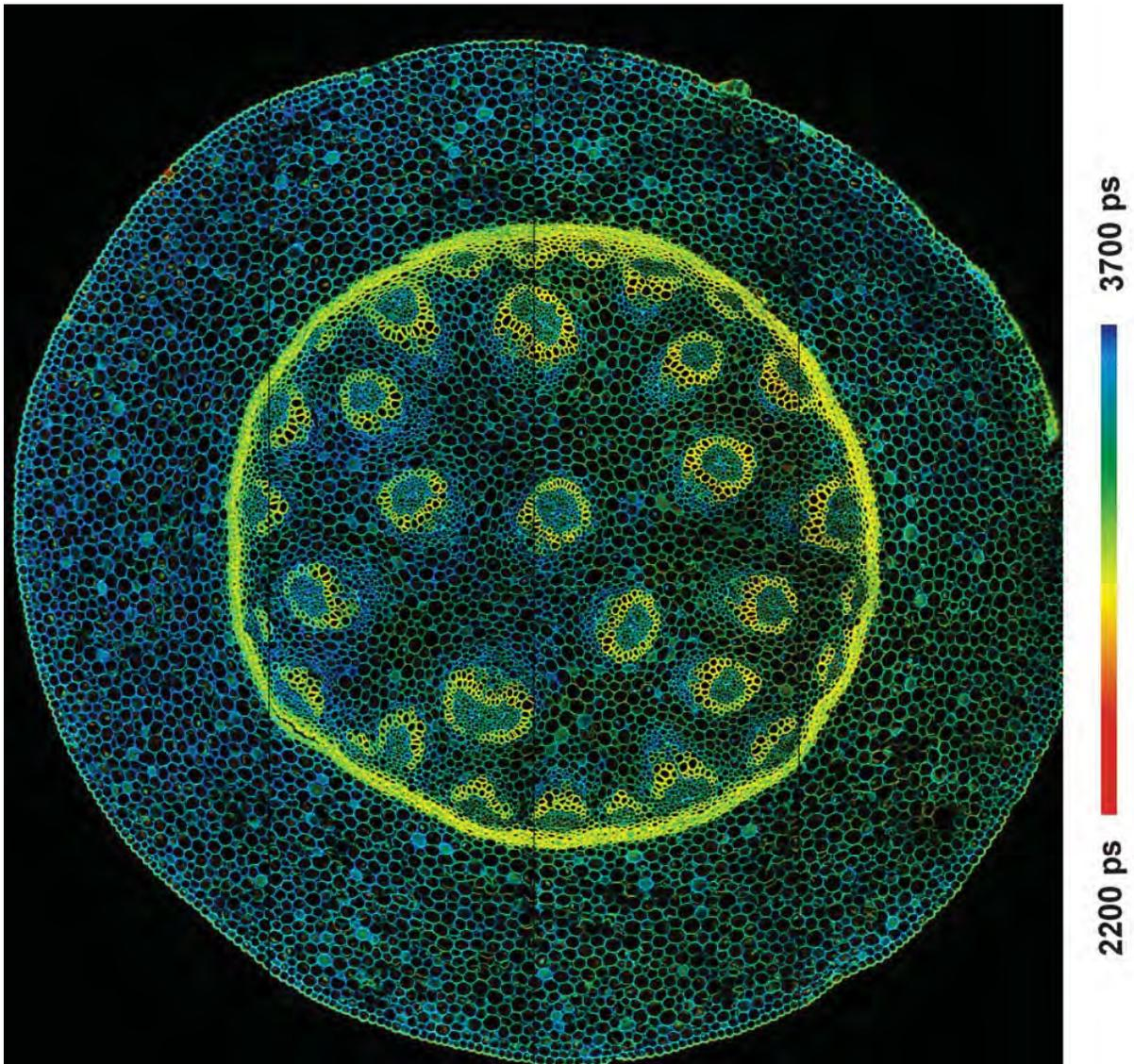
Fig. 20: Mosaic FLIM of a *Convallaria* sample. The mosaic has 4x4 elements, each element has 512x512 pixels with 256 time channels. The complete mosaic has 2048 x 2048 pixels, each pixel holding 256 time channels. Zeiss LSM 710 with bh Simple-Tau 150 FLIM system. Total sample size covered by the mosaic 2.5 x 2.5 mm.
