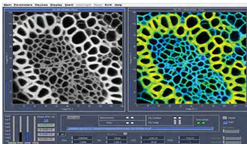
Fig. 10: Fast online FLIM. Intensity image (left) and lifetime image (right). Images 128 x 128 pixels, recorded at a speed of 5 images per second.
