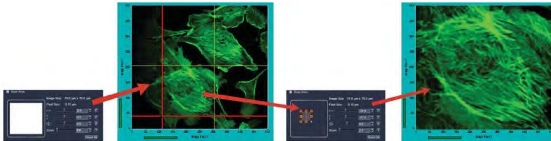
Fig. 7: Interactive scanner control for external microscope software. Example for Zeiss LSM 780/880.
