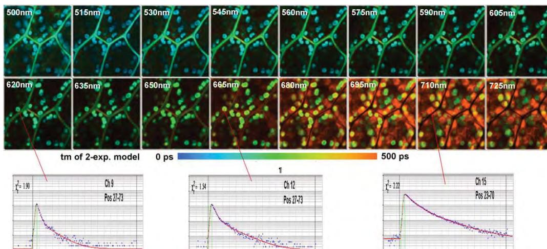
Fig. 17: Multiphoton Multispectral NDD FLIM. Lifetime images and decay curves in selected pixels and wavelength channels. LSM 710 NLO, bh MW FLIM detector
