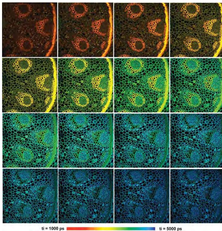
Fig. 14: Multi-wavelength FLIM, 16 images with 512 x 512 pixels and 256 time channels were recorded simultaneously. bh DCS-120 confocal scanner, bh MW-FLIM GaAsP 16-channel detector, Zeiss Axio Observer microscope.
