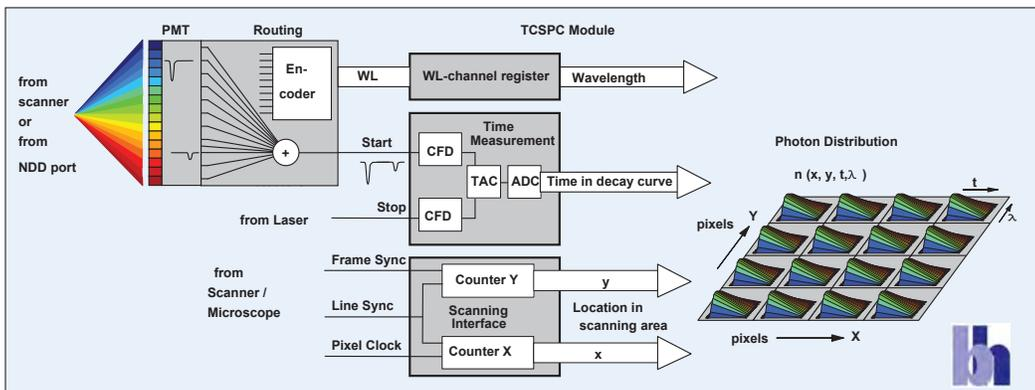
Fig. 2: Principle of Multi-Wavelength TCSPC FLIM
