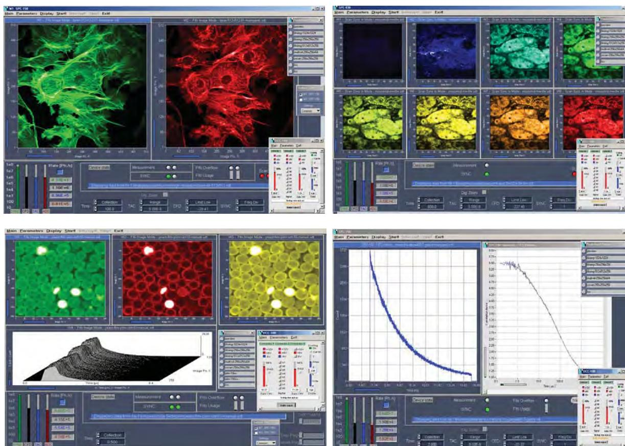
Fig. 4: SPCM software panel. Top left to bottom right: FLIM with two detector channels, multi-spectral FLIM, combined fluorescence / phosphorescence lifetime imaging (FLIM/PLIM), fluorescence correlation (FCS).
