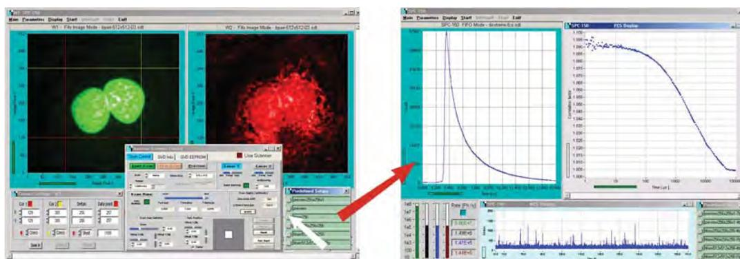
Fig. 6: Changing between different instrument configurations: The software switches from a FLIM configuration into an FCS configuration by a simple mouse click
