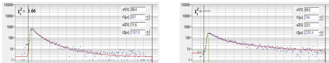
Fig. 16: Decay curves at selected pixel position in the images shown above. Blue dots: Photon numbers in the time channels. Red curve: Fit with a double-exponential model.
