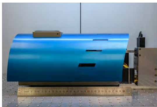
Figure 6 TeraCascade1000 with integrated auto-alignment module at its output.
