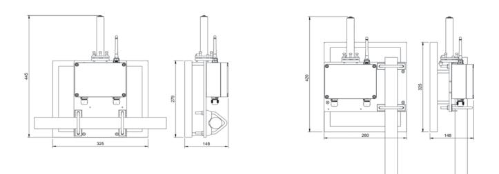
figure 2 dimensions, the drawing on left shows the horizontal (railing) mounting version and the drawing on right shows the vertical (mast) mounting version (as shown in the photo on page 1)
