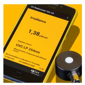
The UV Radiometer SXL 55-UVC is a radiometer / dosimeter for measurement of the germicidal irradiation and dose of a UVC Hg low pressure source at a definded position. It consists of a PTB traceably calibrated UVC sensor and a smartphone.
