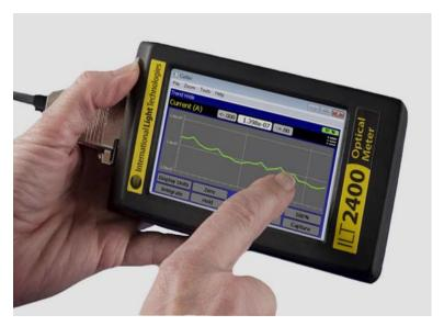
AquiSense Technologies is able to supply the ILT2400 Hand-Held Light Meter by International Light Technologies. It's one of the most advanced devices of its kind on the market today. ILT's Accuspan software automatically sets the averaging while rapidly measuring over 8 decades of light intensities. The internal software allows customers to capture a peak as brief as 100µS and to store up to 16 readings per second. The color display works in both landscape and portrait mode.
