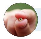
Utilizes small, state of the art UV-C LEDs which provide pathogen reduction without the use of harmful chemicals or mercury-based UV lamps.
