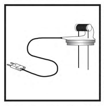
**Construction**: The Type-K Thermocouple sensor is fabricated using special limit error thermocouple wire. This wire is rated at +/-1.1° C. The sensor is applied directly to the coil of the Infrared Light Source. High temperature, low expansion, material is used to apply the sensor to the source. The thermocouple is terminated with a standard Type-K miniature plug. Other thermocouple types can be supplied on request.
