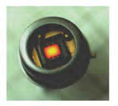
The HawkEye IR-50 pulsed infrared emitter in a TO5 header uses a micromachined source chip with a thin, high-emissivity membrane shown schematically below.
