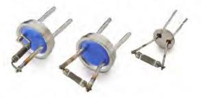
The coiled filament operates at approximately 800°C when powered with 4 watts. The radiating element is a coil of resistance wire which has a high emissivity in the Infrared spectral region. The coil is supported on a cylindrical substrate of alumina. Due to the reduced mass of this unit it can be pulsed at 1 hertz with a resultant temperature variation that can be detected. The unit does not require operation in a sealed atmosphere.
