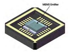
Many filament materials have been used, including traditional metals and polysilicon. MEMS techniques have produced single-crystal silicon filament sources that can operate at 1200 K with 10.7 mW of total radiated power from a 1-mm<sup>2</sup> emitter. Other filament materials used are diamondlike carbon or diamondlike nanocomposites, which are durable and have widely variable electrical conductance properties.
