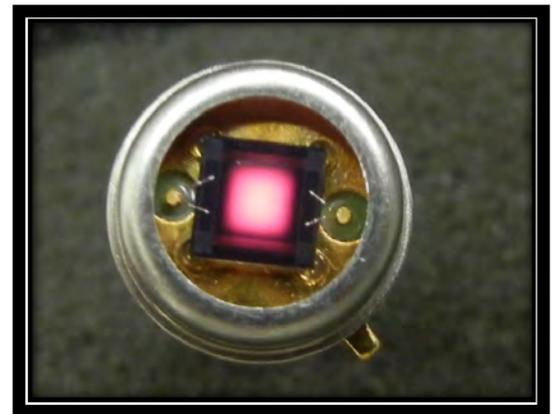
The HawkEye IR-70 pulsed infrared emitter in a TO-39 header uses a micromachined source chip with a thin, high-emissivity membrane assembled using isolation pads for high efficiency and fast response
