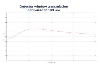
INO MICROXCAM-384i THz Typical AR coating curves
