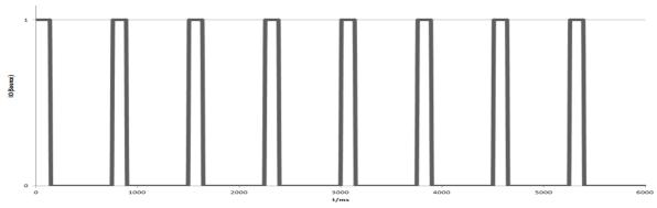
fig. 3 Pulse sequence of the source
