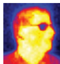
Picture of a face profile, taken with the HTPA32x32d L5.0
