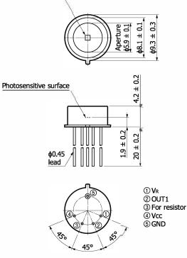
Note: Please connect the same resistance to the terminal @③. Make sure to connect a bypass capacitor (0.1 to 10  $\mu\text{F})$  to the supply voltage ④ to prevent oscillation.
