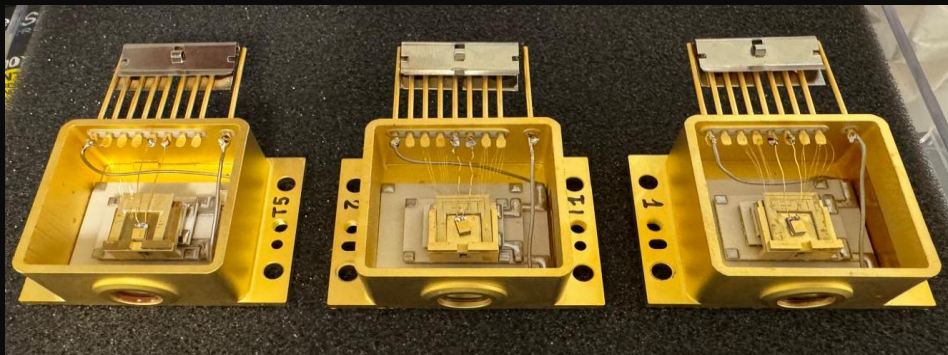
Unsealed HHL housings, 44.5 \times 31.7 \times 19 mm, each carrying a surface-emitting THz QCL.
