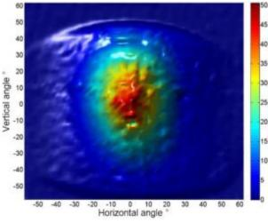
Typical beam profile of an uncollimated QCL.
