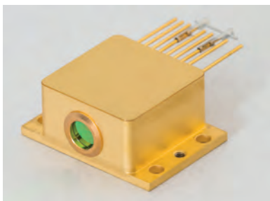
HHL package suitable for higher dissipation CW-DFB
