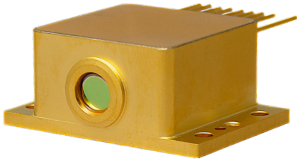
Picture of a HHL with collimated beam output. The lens is inside the housing, protected by a tilted window with AR coating. HHL base to be attached on flat heatsink surface using M3 screws
