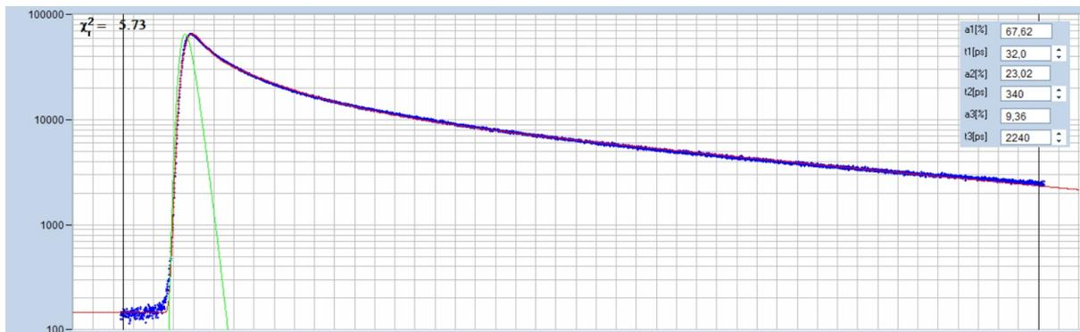
Fig. 2: Triple-exponential fit with SPCImage NG [5], measured in cuvette setup. Decay data from Ardbeg, green curve in Fig. 1. Decay curve shown blue, IRF green, fit with model function red. Horizontal axis 0 to 5 ns, 100 ps per division. The fastest component,  $t_1$ , comes out with a lifetime of 32 ps and an amplitude of 67.6 %.
