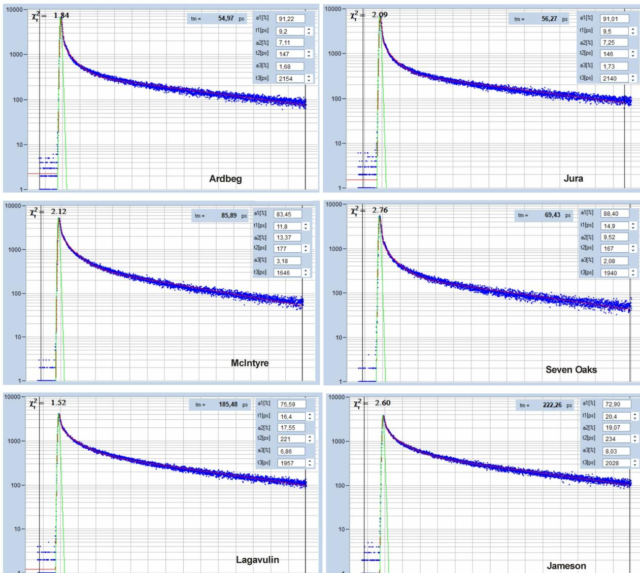
Fig. 4: Decay curves and decay parameters for 6 different brands of Whisky. Two-photon excitation at 780 nm, HPM-100-06 hybrid detector.
