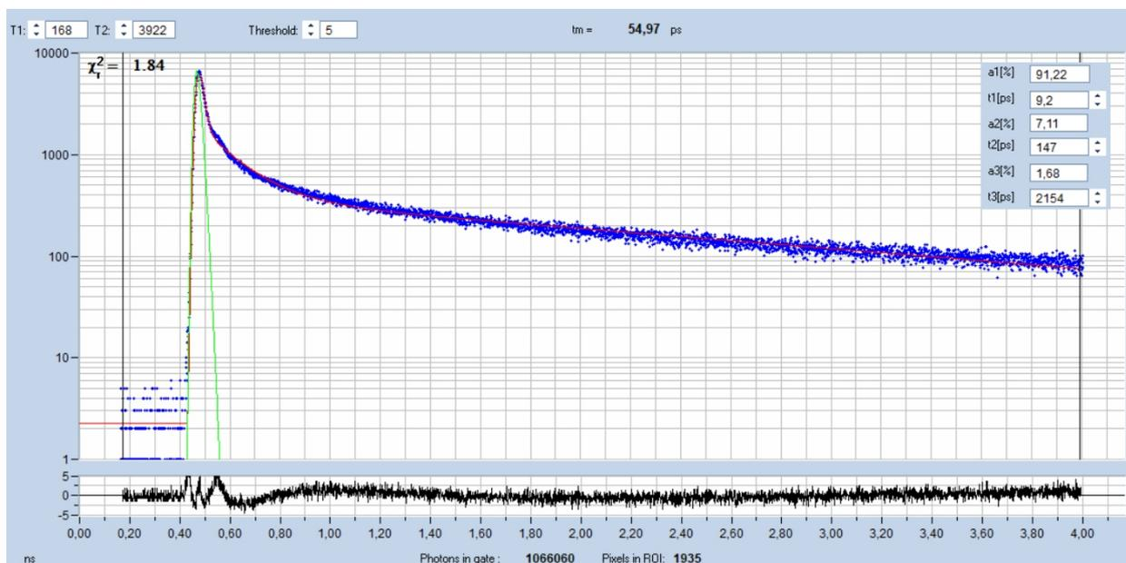
Fig. 3: Two-photon decay curve of Ardbeg Scottish whisky. The fluorescence decay curve is shown blue, the IRF green, and the model function red. The decay parameters are show upper right. The fast decay component,  $t_1$ , has a lifetime of 9.2 ps and an amplitude of 91.2 %.
