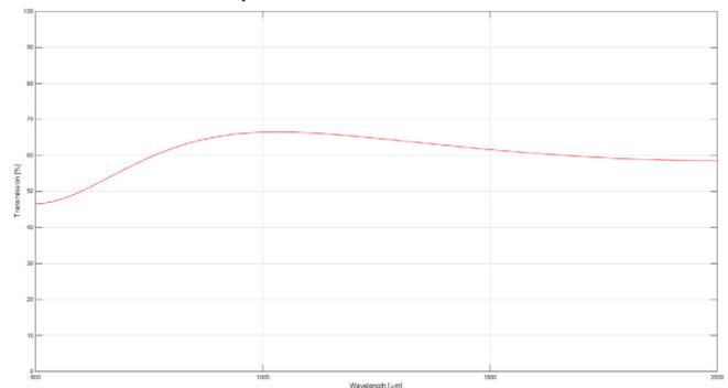
INO MICROXCAM-384i THz Typical AR coating curves
