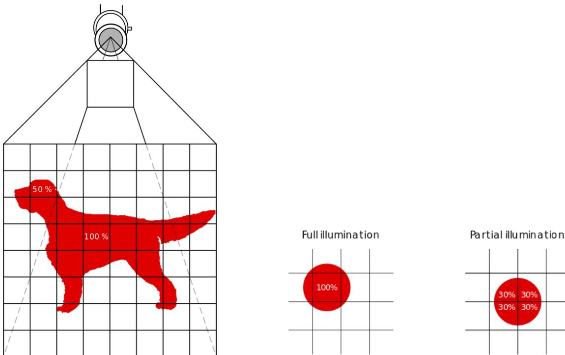
There are two pixels, where the filling factor of the dog versus the background is shown. For the 100% pixel in the middle the camera will detect the temperature of the specific part of the dog. But for the 50% filled pixel at the dog's head the camera will measure the superposition of the dog's head temperature and the background.
