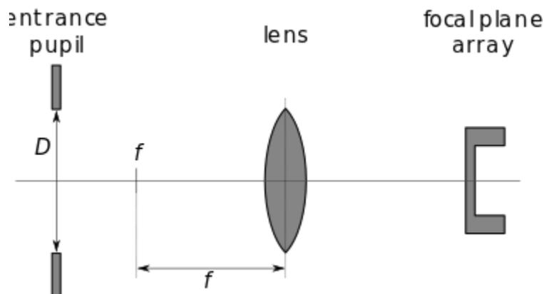
In general, a smaller f-number corresponds to more radiation that can reach the sensitive matrix of the FPA. More radiation will result in a better signal to noise ratio (SNR). Because a low f-number requires a lens system with larger diameter, it also requires more material, and tighter manufacturing tolerances. Better performance is therefore only achievable at a higher price.
