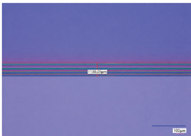
Figure 6. Top-down optical micrograph of the wafer edge exposure region, showing interference fringe structure at the resist boundary. The measured fringe spacing corresponds to an approximate slope of the exposure transition.
