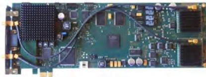
**SPC-160PCIe TCSPC Module with PCI Express Interface**
