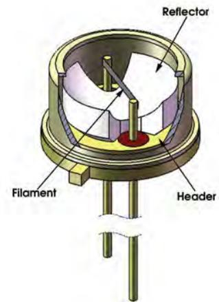
Reflectors often are used – as with the wound filament emitters – to direct all possible radiation out of the package, particularly in vertically oriented filaments.
