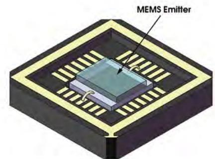
Many filament materials have been used, including traditional metals and polysilicon. MEMS techniques have produced single-crystal silicon filament sources that can operate at 1200 K with 10.7 mW of total radiated power from a 1-mm<sup>2</sup> emitter. Other filament materials used are diamondlike carbon or diamondlike nanocomposites, which are durable and have widely variable electrical conductance properties.
