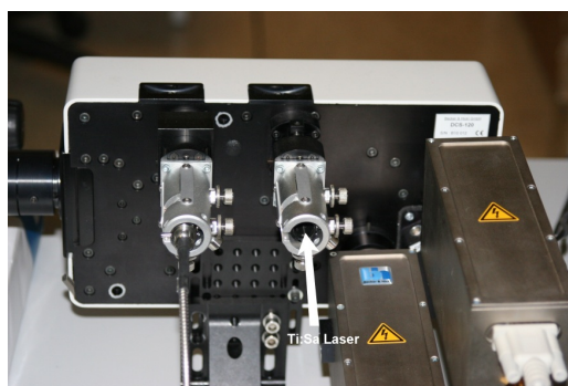
Fig. 344: Input of a Ti:Sa laser into the DCS-120 scanner
