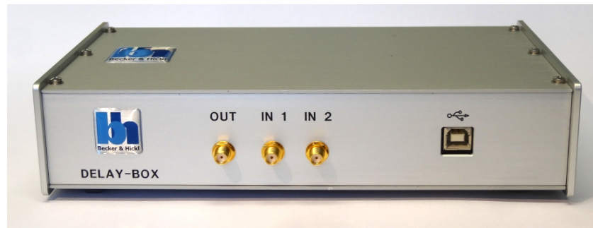
Fig. 108: Delay switch box. It is used to set the correct temporal relationship between the detector signals and the synchronisation signals from the lasers. The correct Sync delay for different system configurations is set by loading setup data via the SPCM software.
