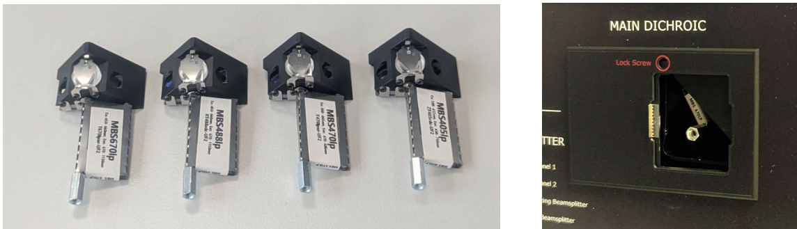
Fig. 83: Left: Main dichroic beamsplitter assemblies for different wavelength. Right: The beamsplitter assembly is located behind a flap in the cover of the scan head.
