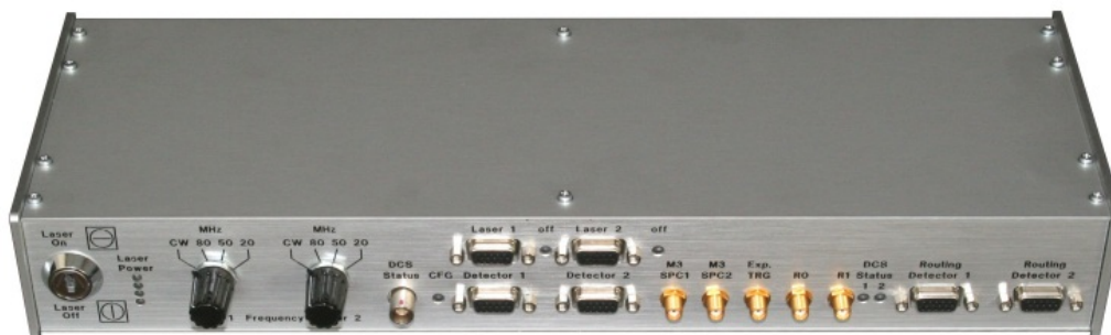
Fig. 106: DCS switch box
