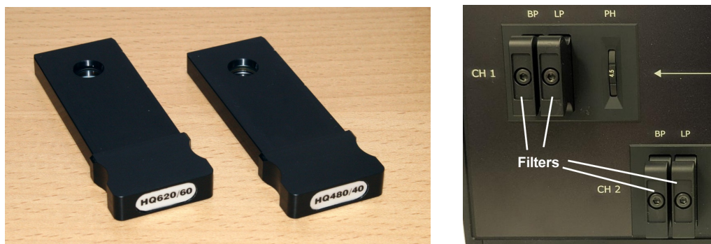
Fig. 88: Emission filters. Left: Filter sliders. Right: Filter positions in DCS-120 scan head
