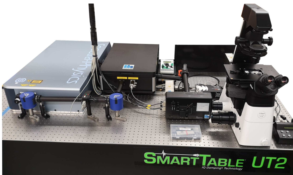
Fig. 12: DCS-120 Super MPC system. Multiphoton FLIM by Ti:Sa laser combined with tuneable confocal FLIM via SHG of Ti:Sa laser
