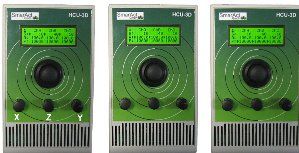
Fig. 92: Piezo hand controller in step width selection mode (left) and voltage selection mode (middle), and speed selection mode (right)
