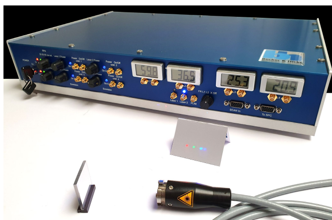
Fig. 99: LHB-104 Laser Hub, with four lasers of 405 nm, 488 nm, 515 nm, and 640 nm. The photo shows 4-wavelength output from a single fibre. For demonstration, the beams were separated by an optical grating.
