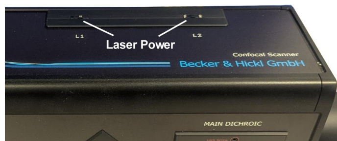
Fig. 81: Optical power control wheels at the DCS-120 scan head
