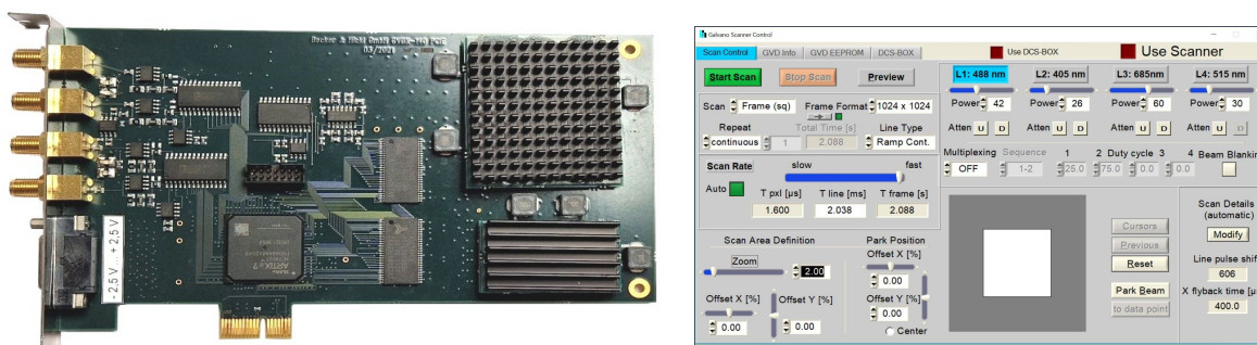
Fig. 95: GVD-140 Scan controller card. The card controls the scanner and four lasers. Software panel shown on the right.
