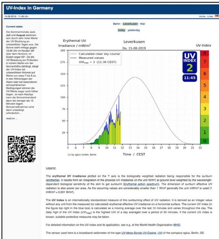
figure 3 example of the web based desktop display, colors and UV Index calculation according to the WHO requirements
