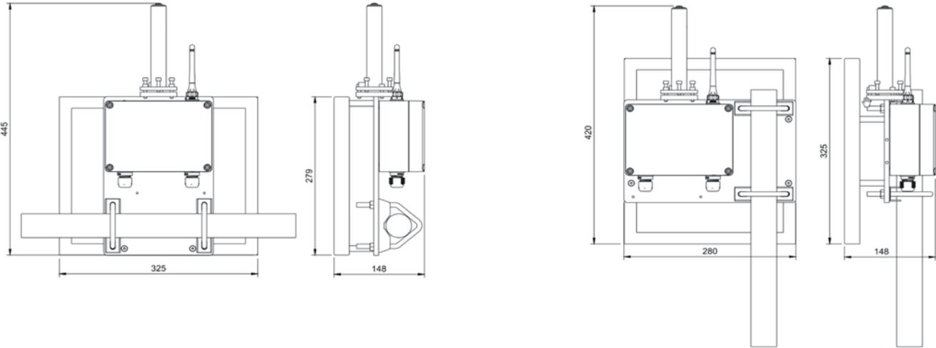
figure 2 dimensions, the drawing on left shows the horizontal (railing) mounting version and the drawing on right shows the vertical (mast) mounting version (as shown in the photo on page 1)
