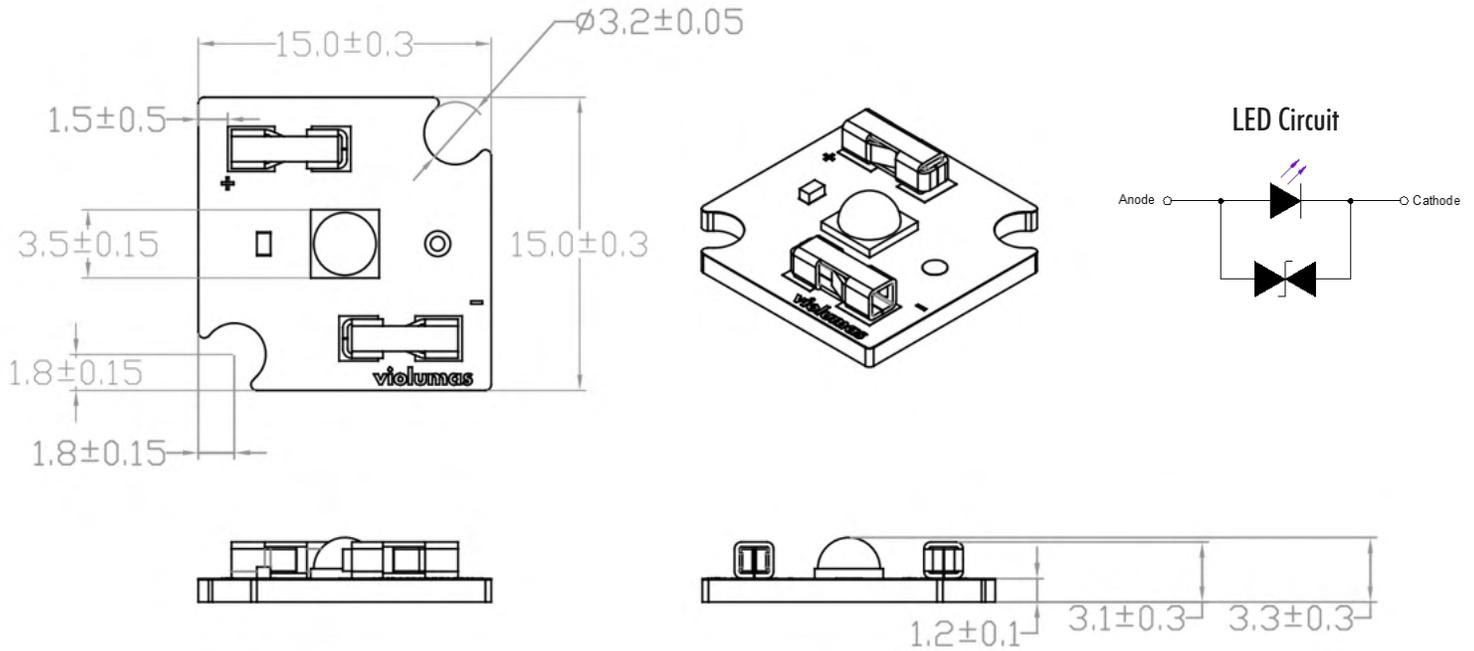
Note: The maximum offset (tolerance) for lens alignment over the LED is 0.2mm.
