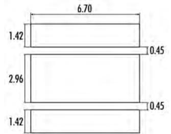
Note: The maximum offset (tolerance) for lens alignment over the LED is 0.2mm.
