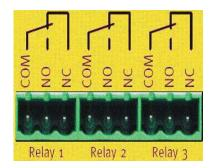
Three potential-free relays can be used for process control.
