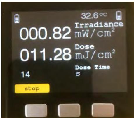
The current dose and the time elapsed since the dose measurement start is displayed. The dose measurement can be stopped while pressing the stop button.
