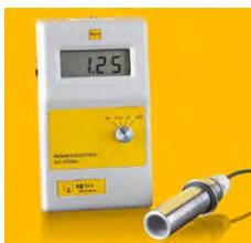
Reference Radiometer for validation of DVGW-40° duty sensors according to DVGW W 294-3:2006. The unit is powered by a 9 V battery that allows several years of use if infrequently used. The radiometer price includes a PTB traceable calibration.
