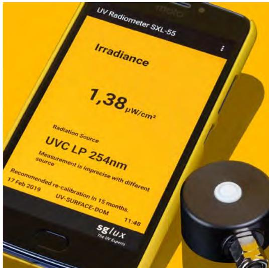
The UV Radiometer SXL 55-UVC is a radiometer / dosimeter for measurement of the germicidal irradiation and dose of a UVC Hg low pressure source at a defined position. It consists of a PTB traceably calibrated UVC sensor and a smartphone.
