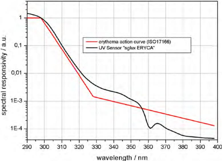
figure 1 spectral responsivity of the sglux ERYCA sensor compared with the erythema action curve according to ISO17166:2019
