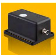
Rugged UV datalogger for long-term monitoring of moving goods, persons or animals. It includes one or two customized UV sensors (broadband UV, UVA, UVB, UVC, erythema or  $v(\lambda)$ ) with PTB traceable calibration. Additional sensors for temperature, pressure, relative humidity, and illuminance (VIS) are available. The UVMiniLog stores up to 2,000,000 data records. The battery lifetime is up to 18 months of permanent logging without re-charging of the battery.
