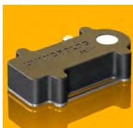
Rugged UV datalogger for long-term monitoring of moving goods, persons or animals. It includes one customized UV sensor (broadband UV, UVA, UVB, UVC, erythema or  $v(\lambda)$ ) with PTB traceable calibration. Additional sensors for temperature, pressure, relative humidity, and illuminance (VIS) are available. The UVMicrolog stores up to 2,000,000 data records and is also available in an IP67 waterproof version.
