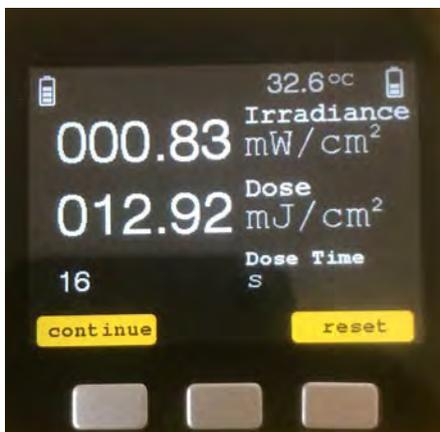
After having stopped the dose measurement it is possible to continue (press the "continue" button) or to reset (press the "reset" button) the dose measurement. After resetting the dose measurement the "start" button re-appears.
