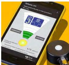
Digital Smartphone (Android) based UV Index radiometer with graphic display for hazard assessment of natural UV radiation in workplaces according to the ISO 17166 standard (UV Index). The price includes a UV sensor with PTB traceable calibration, a calibration certificate and a Smartphone. The radiometer is also available without a Smartphone and a software download.
