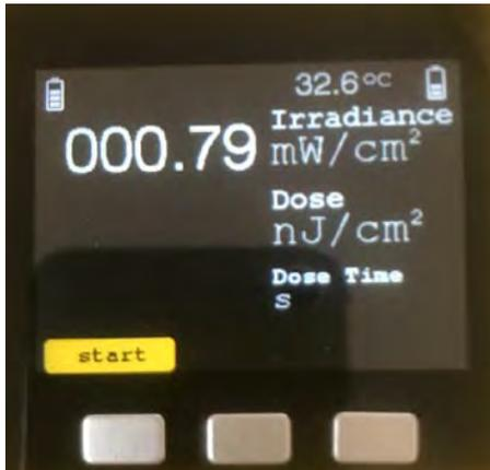
The receiver starts displaying the current irradiance. While pressing the "start"-button a dose measurement can be started.
