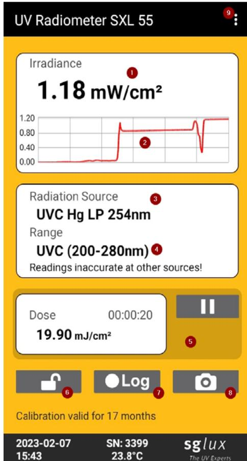
(5) All functions for dose measurement are located here. The dose is the integration of the irradiance over time. If a dose measurement runs over a very long period of time, the unit changes (in the picture e.g. from  $\text{mJ}/\text{cm}^2$  to  $\text{J}/\text{cm}^2$ ). On the picture the measurement has been started 20s ago. This can be stopped with the pause function. The characters "Play" and "Repeat" then follow, with which the measurement can be continued (Play) or reset (Repeat).
