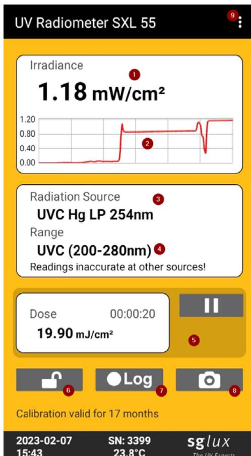
(1) Display of irradiance with the area unit  $\text{cm}^2$ . The displayed irradiance unit is specified by the measuring range of the sensor and can be  $\text{nW}/\text{cm}^2$ ,  $\mu\text{W}/\text{cm}^2$ ,  $\text{mW}/\text{cm}^2$ , or  $\text{W}/\text{cm}^2$ .
