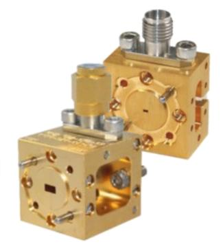
Lytid's range of high power frequency multipliers provide state-of-the-art performances across the sub-terahertz band. These frequency doublers are commonly used to extend the frequency range of microwave and mmW sources towards higher frequencies. The doublers are based on planar GaAs Schottky diode technology
