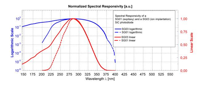
Broadband SiC based UV photodiode A = 1.0 mm<sup>2</sup> with VUV responsivity
