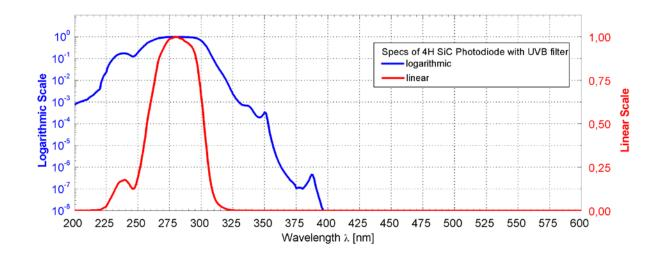
UVB-only SiC based UV photodiode A = 0,06 mm<sup>2</sup>
