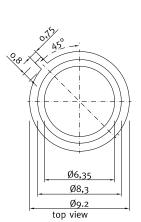
Concentrator lens SiC based UV photodiode A = 1,0 mm<sup>2</sup>
