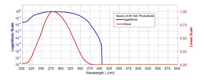
Broadband SiC based UV photodiode A = 1,82 mm<sup>2</sup>
