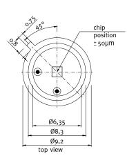
Broadband SiC based UV photodiode A = 1,82 mm<sup>2</sup>
