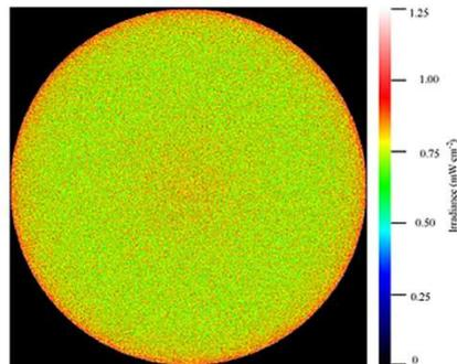
Typical 285nm Irradiance at the end of the collimating tube
