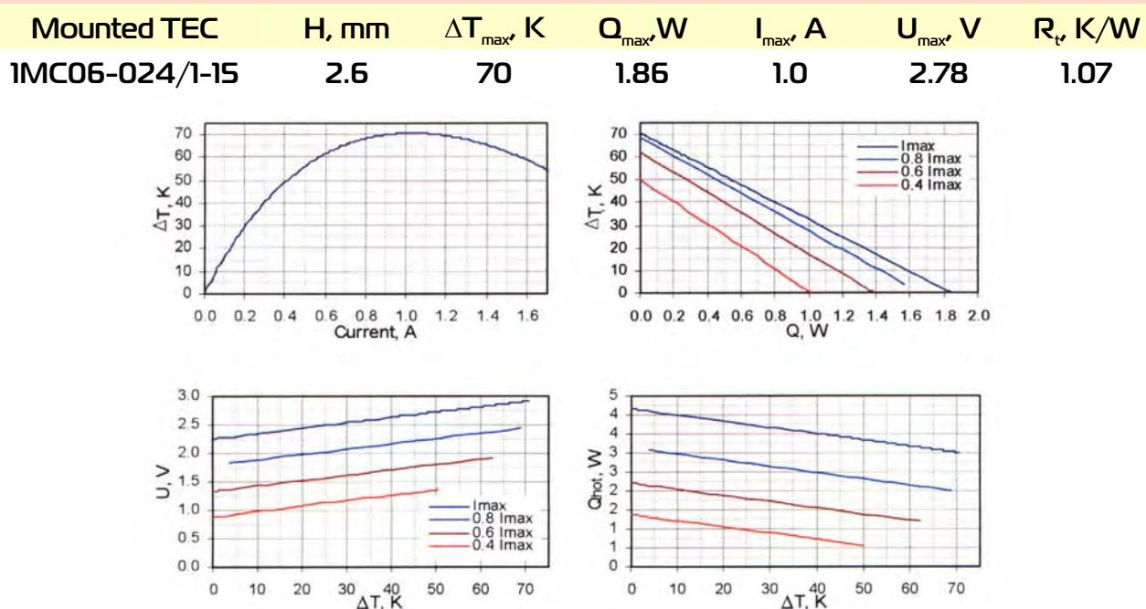
Data for  $T_{hot}=300$  K, from [www.tec-microsystems.com](http://www.tec-microsystems.com); [www.rmtltd.ru](http://www.rmtltd.ru)
