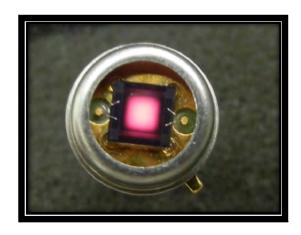
The HawkEye IR-70 pulsed infrared emitter in a TO-39 header uses a micromachined source chip with a thin, high-emissivity membrane assembled using isolation pads for high efficiency and fast response
