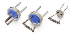
The coiled filament operates at approximately 800°C when powered with 4 watts. The radiating element is a coil of resistance wire which has a high emissivity in the Infrared spectral region. The coil is supported on a cylindrical substrate of alumina. Due to the reduced mass of this unit it can be pulsed at 1 hertz with a resultant temperature variation that can be detected. The unit does not require operation in a sealed atmosphere.
