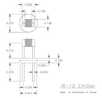
The coiled resistance wire filament IR-12 operates at 825°C (1100K) when powered with 4.5 volts @ 1.8 amps (8 watts). The IR-12K takes higher electrical power and runs hotter. Emissivity is ~80% in the IR. The coil is wound on a cylindrical alumina substrate. Generally the IR-12K is recommended for maximum versatility. Operation in a controlled or sealed atmosphere is not required for either device.
