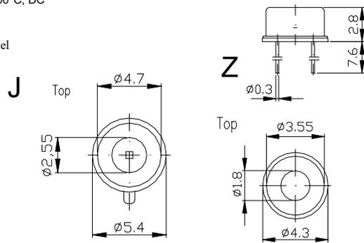
Filter types for temperature measurements
