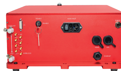
GLIDER back side showing controls and connectors
