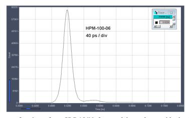
Fig. 8: Instrument response function of an SPC-154N four-module package with the Photon Spinner and an HPM-100-06 hybrid detector. FWHM is 22.6 ps.
