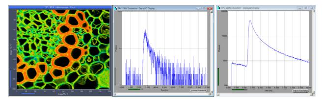
Fig. 3: FLIM of a Convallaria sample. Acquisition time 250 ms, 256x256 pixels, 1024 time channels, time channel width 12 ps. Middle and right: Decay curve in 4x4 pixel area and decay curve over entire image. DCS-120 system with 488 nm diode laser and HPM-100-40 detector.
