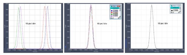
Fig. 7: Electrical IRFs of the four SPC-150N modules. Before (left) and after delay alignment (middle). The combined IRF of the four SPC-150N is shown on the right. The FWHM of the combined IRF is 6.8 ps.
