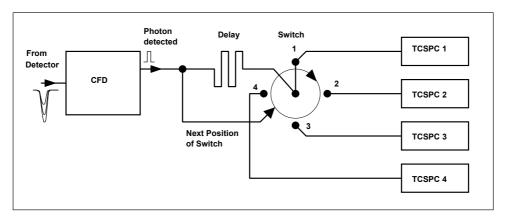
Fig. 1: The 'Photon Spinner'. Every photon puts the position of a signal switch forward by one position. It arrives at the switch shortly after the switching action is complete, and proceeds into the next TCSPC module. Because the time between the switch set and the arrival at the switch is constant the switching transient has no effect on the photon timing.
