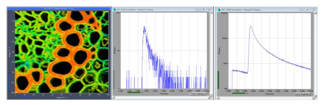
Fig. 2: FLIM of a Convallaria sample. Acquisition time 100 ms, 128x128 pixels, 1024 time channels, time channel width 12 ps. Lifetime range 1 ns (red) to 2.5 ns (blue). Middle and right: Decay curve in 5x5 pixel area and decay curve over entire image. DCS-120 system with 488 nm diode laser and HPM-100-40 detector.
