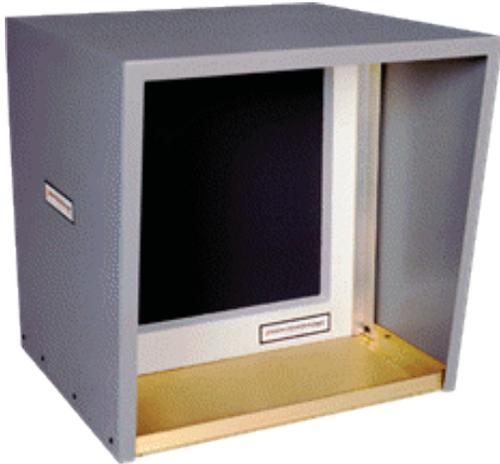
Our extended area sources are flat plate emitters with special high emissivity coating providing 0.96 average emissivity. Extended area sources provide large target with high radiant intensity for application where a cavity blackbody is too small.
