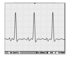
Fig. 1: Left: APS-100 photodiode module. Right: Output pulses for an 80 MHz laser pulse sequence.
