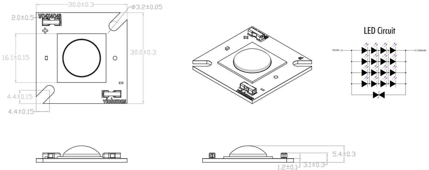
Note: The maximum offset (tolerance) for lens alignment over the LED is 0.2mm.
