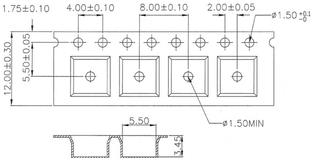
Each reel is loaded with 350 units and includes a leader section (200mm) and a trailer section (200mm) with empty pockets. The diameter of the reel is 177.8mm. Devices are placed with the anode to the left.
