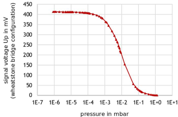
The above curve shows the sensitivity of a relatively large chip (HVS 03k) with  $4 \times 4 \text{ mm}^2$  chip size. You can combine this with a second, smaller chip with  $1 \times 1 \text{ mm}^2$  which has its peak sensitivity in higher pressure regimes. This combination of two chips allows to sense the whole pressure range from atmospheric pressure down to  $10^{-6}$  mbar.
