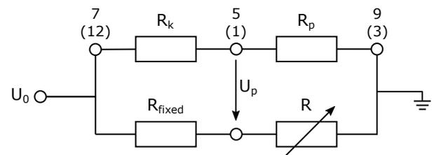
One possible readout is the wheatstone bridge arrangement. The output voltage  $U_p$  should be balanced ( $U_p = 0$  V) at atmospheric pressure (1013 mbar) by using the potentiometer  $R$ . The resistance  $R_p$  is changing with pressure  $p$  and therefore  $U_p$  is changing as well.
