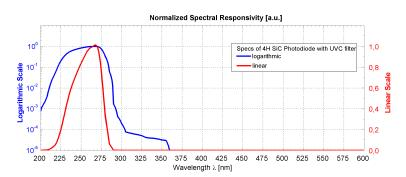
• Spectral sensitivity from 225 to 287 nm, peak wavelength 275 nm, according to DVGW W294/3 and OENORM M5873, different packaging, sorted by detector areas.
