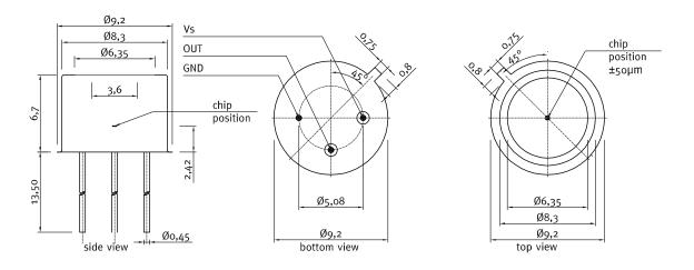
UVA-only SiC based UV photodetector with integrated amplifier
