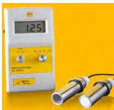
Reference Radiometer with two sensors for validation of DVGW-40° and ÖNORM-160° duty sensors according to DVGW W 294-3:2006 and ÖNORM M 5873. The unit is powered by a 9 V battery that allows several years of use if infrequently used. The radiometer price includes a PTB traceable calibration.
