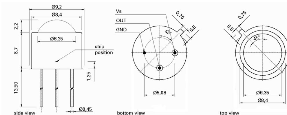
TOCON in TO5 housing with lens cap
