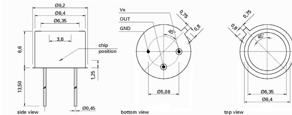
TOCON in TO5 housing with filter, diffusor and / or attenuator
