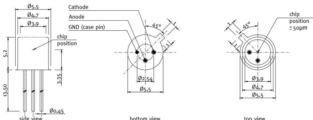
Selection code “18ISO90” → TO18 Ni plated housing, 5.5 mm diameter, 5.2 mm height three gold plated pins (Anode and Cathode isolated, additional third pin for optional grounding of the body).
