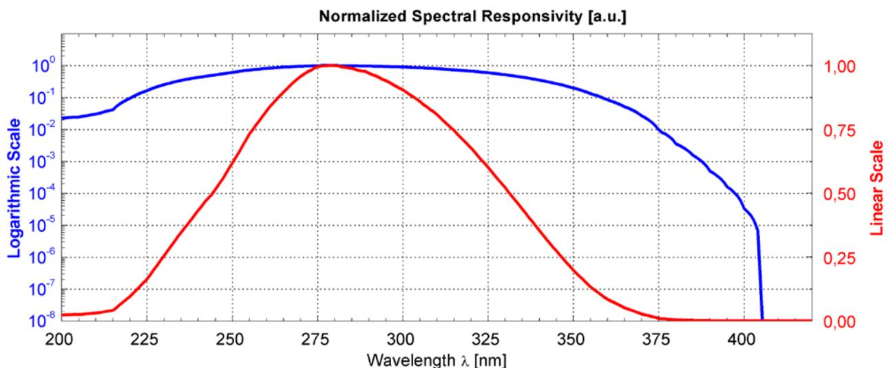
The curve's maximum is at approximately 280 nm. The response falls down to 10% of maximum at 221 nm, (UVC edge) and 358 nm, (UVA edge). Unfiltered SiC is the standard application and can be used for any UV measurements where the whole UV band needs to be measured or a quasi monochromatic UV source (such as low pressure lamps) is controlled.
