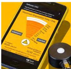
Radiometers for hazard assessment of artificial UV radiation emitted by low pressure UVC sources in workplaces, according to European Union guideline 2006/25/EC, visualization of the maximum exposure time per day, with acoustical and optical warning features.
