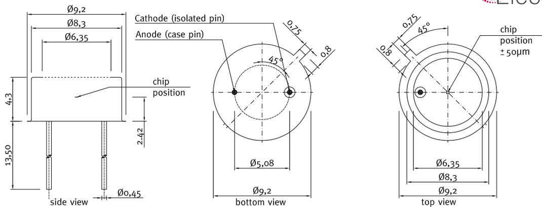
Selection Code "5" (photodiodes without filters) → TO5 Ni plated housing, 9.2 mm diameter, 4.3 mm height, two gold plated pins (Anode grounded and Cathode isolated).
