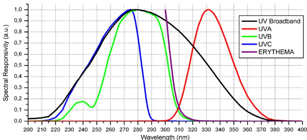
The graph assigns the filtered photodiode’s spectral response to an individual wavelength. The following table extracts the most important specifications.
