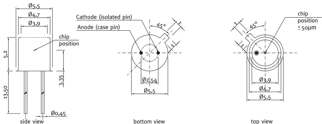
Selection code “18” → TO18 Ni plated housing, 5.5 mm diameter, 5.2 mm height two gold plated pins (Anode grounded and Cathode isolated).
