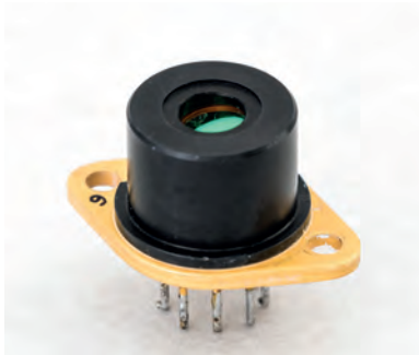
TO3 package suitable for lower dissipation CW-DFB
