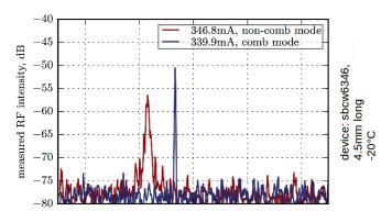
RF Spectrum of a Frequency Comb laser showing comb operation at an operating current of 339 mA
