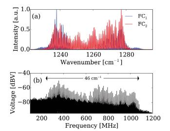
Top: Overlapping optical spectra of two typical Frequency Comb
